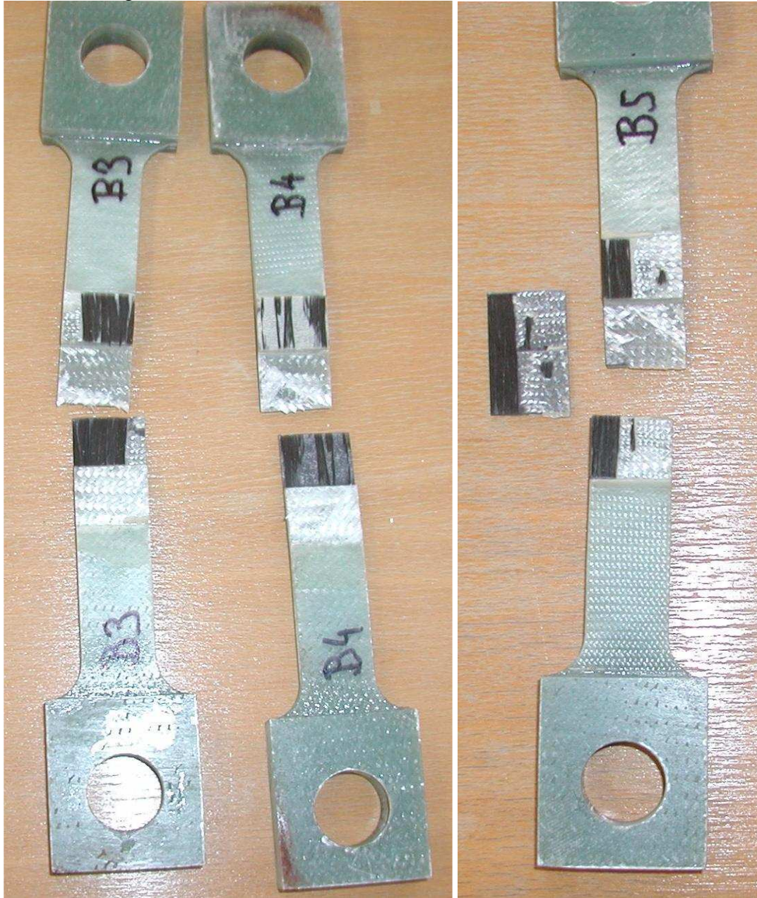
Figure 5: Specimens after fatigue tests.
